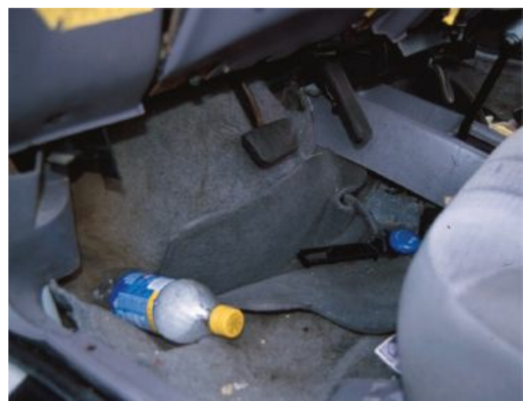
FIGURE 2 • Interior damage with >12 in of toepan intrusion into the driver's space. This meets step 3 (Mechanism of Injury) criteria for field triage and is associated with significant risk of severe injury.
