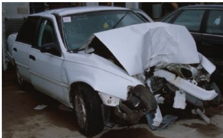
FIGURE 1 • Vehicle damage from frontal crash into large tree.
